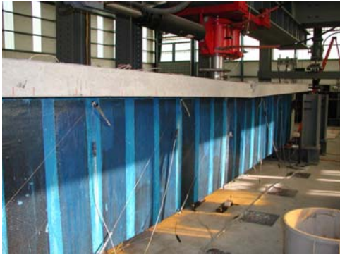
Above: CFRP strengthened beam control specimen; approximately 500,000 pounds of applied force was used to fail the specimen.
