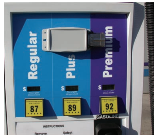
In the Oregon mileage fee concept, mileage data is downloaded at the fuel pump using an on-vehicle device that identifies miles driven within various pre-identified zones (above). Fee collection occurs at a fuel pump outfitted with mileage reading equipment (below).
